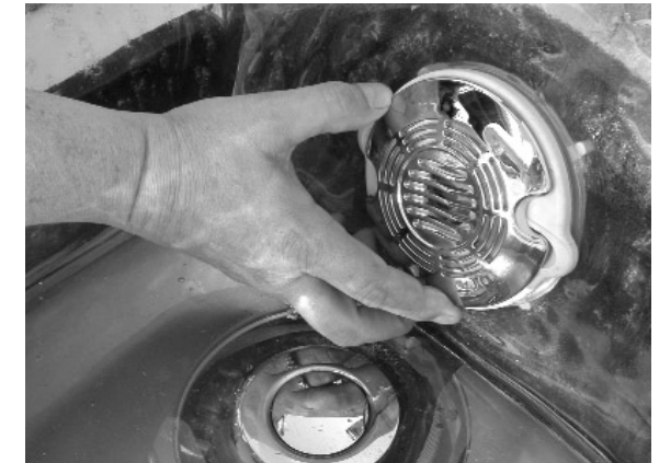
Replace screen by turning clockwise
